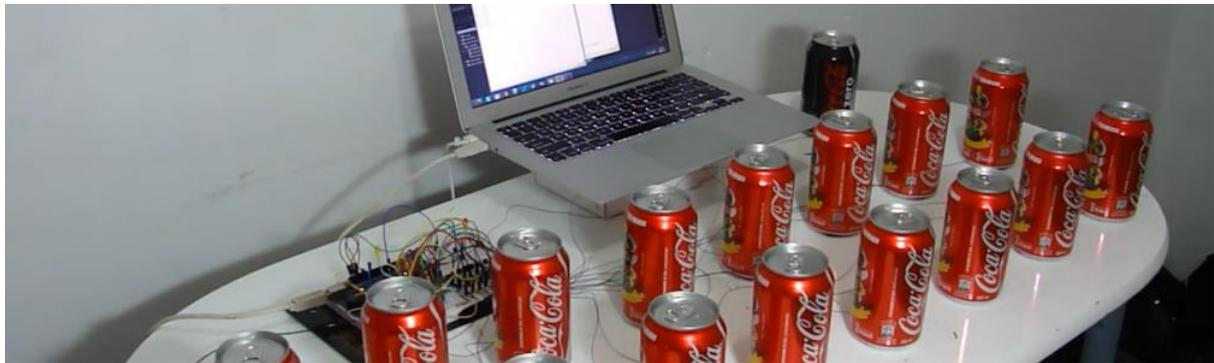
Each can is connected to the BC548B transistor, which essentially amplifies the signal from the body when the can is touched. The Arduino reads the signal from the transistor and converts it to a note sent to your computer through a serial connection.
